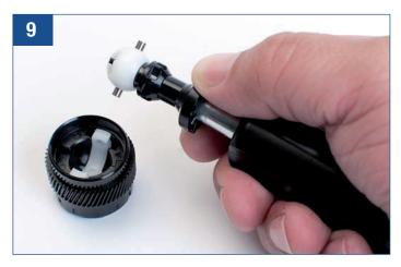
With the cradle attached to the gear, *(Photo 10)* shows how the Drum Axle Tool (Article #61077) is used to position the axle into the receiving ports of the cradle.
