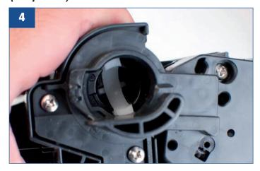
The following pictures will merely illustrate how the drive axle interacts with the gear of the OPC for HP P3015 (Article #19607). The final step will be to use the Drum Axle Tool (Article #61077) to attach the OEM drive axle to the gear of the OPC for HP P3015 (Article #19607) (See photos 5-10).
