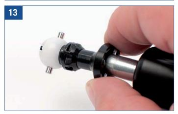
**STEP 5:** With the cartridge fully rebuilt, gently slide the axle into the receiving ports of the OPC for HP P3015 (Article #19607) gear and apply a slight turn counterclockwise until the gear unlocks into place. By holding the newly built cartridge in an upright, vertical orientation, it takes very little effort to secure the axle into the new gear *(See photos 14 & 15).*
