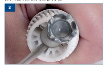
**STEP 4:** Rebuild the cartridge per the remanufactturing guide. For reference, the following picture shows the new Drum Axle Tool article # 61077 before it is built into the new cartridge. Note the slots in the gear that will accept the metal pins from the hub of the drive axle (*See photo 4*).
