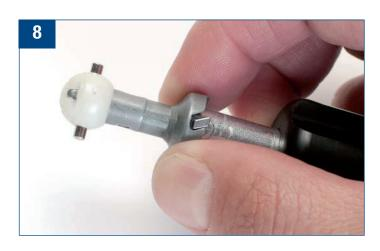
**STEP 6:** Gently slide the axle into the slots of the Drum Axle Tool article #61077 and apply a 1/4 turn counterclockwise until the gear locks into place (See photo 9).
