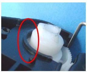
reduce height of the rib to 1.7 mm
