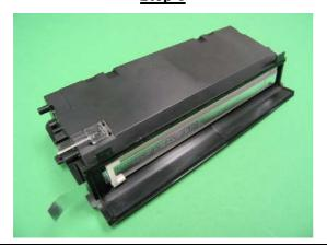
Fit the Hopper Seal on the OEM Toner Hopper Section, and put in the Seal Exit Port Plug. Install the toner.
