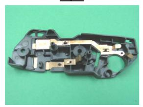
Reassembly the OEM Outer Left End Cap Cover Contact Plates onto the Delacamp HP4700 Outer Left End Cap Cover.
