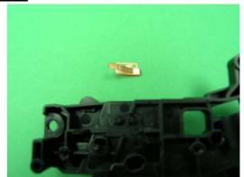
Take off the Contact Plates from the OEM Inner Left End Cap.
