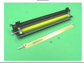
Unscrew the Doctor Blade from OEM Supply Roller Housing Section. Clean the Doctor Blade. Reassemble the Doctor Blade on to OEM Supply Roller Housing Section.
