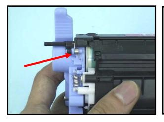
8. Take the OPC drum shutter from the OEM cartridge and fit to the Waste Section. Finally, insert the OPC Drum Shutter Spring. A spare spring is included with the kit.
