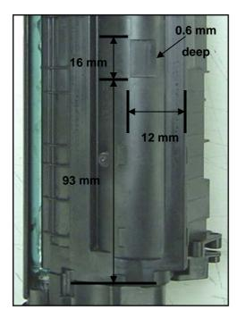
The detail position of the small flat area is show on left picture. This can be done by locating the area within a small fixture and filing off the plastic to create the flat area (0.6 mm deep).
